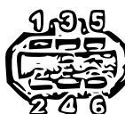
Link Cable / Link Port Pins Numbers
